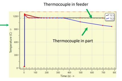
**Summary:** The modified feeder and neck dimensions resulted into elimination of shrinkage defect observed at shop floor. .
