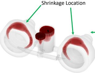
Shrinkage porosity analysis shows micro porosity observed in the different locations of casting and macro porosity at the feeders matching exactly to the shop floor defect.
