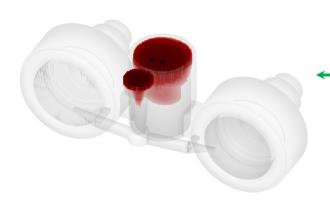
Shrinkage porosity results shows macro porosity in the feeder and there is almost no shrinkage in casting observed at locations of shop floor. Casting is free from shrinkage defect.
