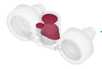
Liquid fraction analysis shows last solidifying metal present in feeder, while there is no liquid metal remaining at the end of solidification in part which gives defect free casting
