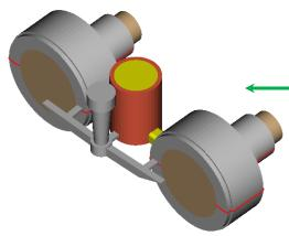
Solidification simulation shows that the feeder neck size is inadequate, and results in shrinkage porosity exactly matching with the defect found in actual casting.
