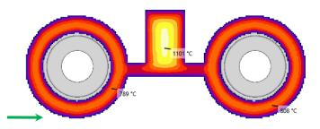
Liquid fraction analysis displays liquid metal remains inside the casting till the end of solidification. The isolated liquid metal is present in the thick regions.
