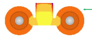
Solidification temperature shows the directional solidification with hottest region in feeder and part connected to feeder at relatively lower temperature.
