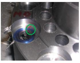
Wall thickness analysis shows a heavy section with 29 mm thickness below L-junction.
